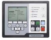
An integrated microprocessor based generator set control system providing voltage regulation, engine protection, alternator protection, operator interface and isochronous governing. Refer to document S-1570 for more detailed information on the control. **AmpSentry** – Includes integral AmpSentry protection, which
