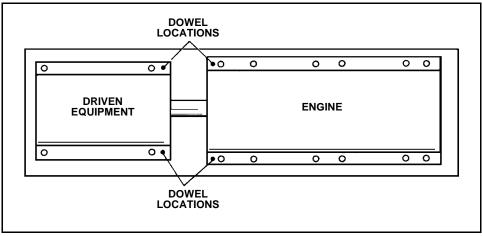
Figure 3-45 Dowel Placement
