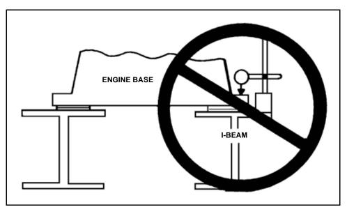
Figure 3-6 Incorrect Mounting
