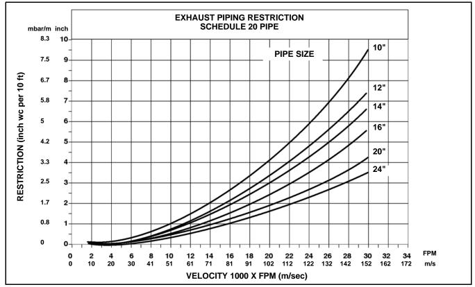
Figure 8-4 Restriction vs. Velocity for Pipe Diameter Up to 24 in.
