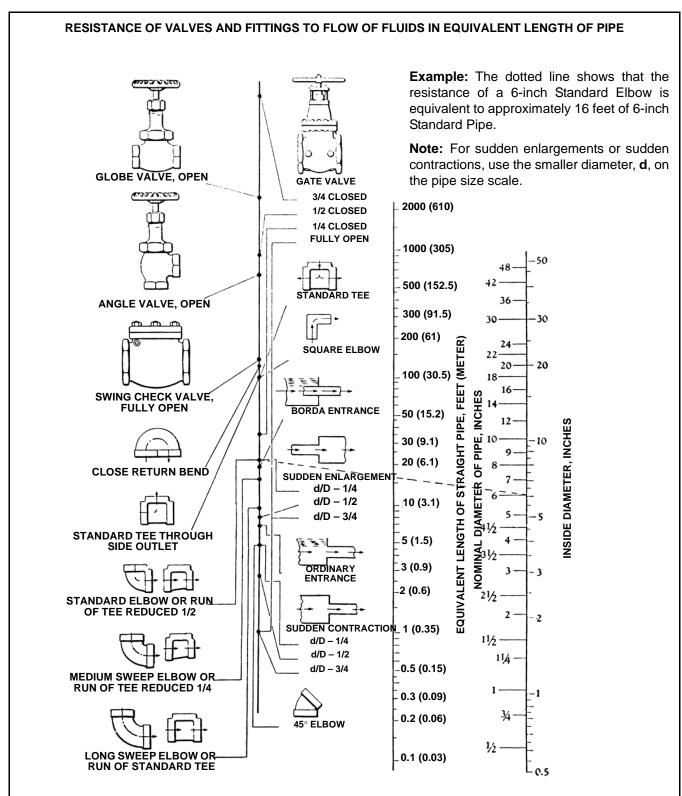
From Crane Co. Technical Paper No. 409. Data based on the above chart are satisfactory for most applications. REPRINTED WITH PERMISSION OF CRANE VALVE GROUP.
