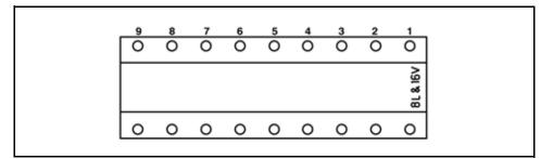
Figure 10-3 Bolt Locations for 16-Cylinder Models
