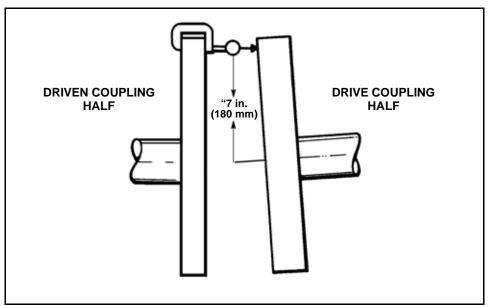
Figure 10-7 Distance from Center of Shaft to Dial Indicator
