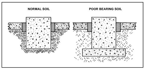
Figure 2-3 Footing for Poor Bearing Soil
