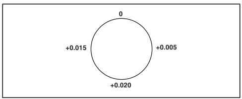
Figure 3-44 Total Indicator Reading (TIR)
