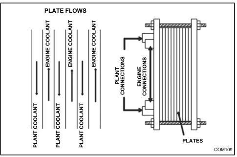
Figure 5-4 Plate-Type Heat Exchanger
