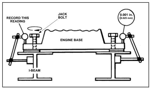
Figure 3-9 Record the Left Free Corner Indicator Reading
