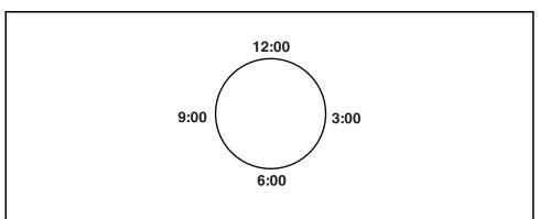
Figure 3-35 Dial Indicator Reading Positions When Measuring Angular Alignment
