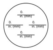
9. Check and adjust parallel alignment. Maximum 0.005 in. (0.127 mm) TIR.
