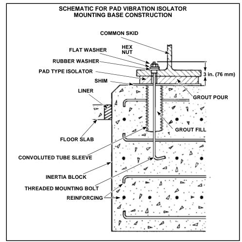
Figure 2-7 Common Skid Mounted on Pad Type Vibration Isolators
