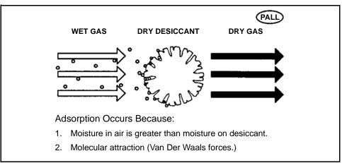
Figure 9-13 Adsorption Drying
