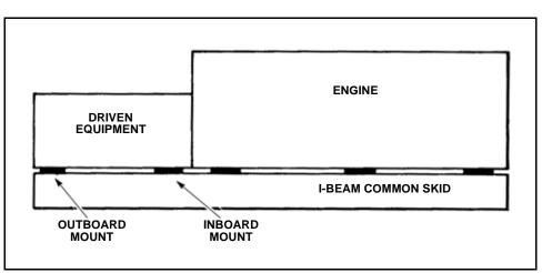
Figure 3-29 Add or Remove Shims from the Mounts on Each End of the Machine to Make Vertical Adjustments
