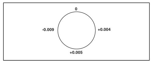
Figure 3-36 Total Indicator Reading (TIR)
