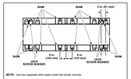
Figure 3-3 Engine Shimming Procedure
