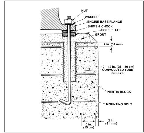
Figure 2-11 Cross Section of Mounting Using Sole Plates
