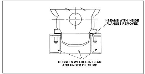
Figure 10-8 Engine Mounted Directly Above Web
