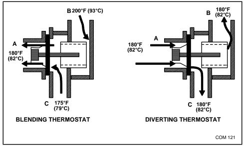
Figure 5-17 Blending and Diverting Thermostats
