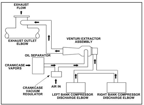
Figure 6-4 Ejector Type System (Standard)
