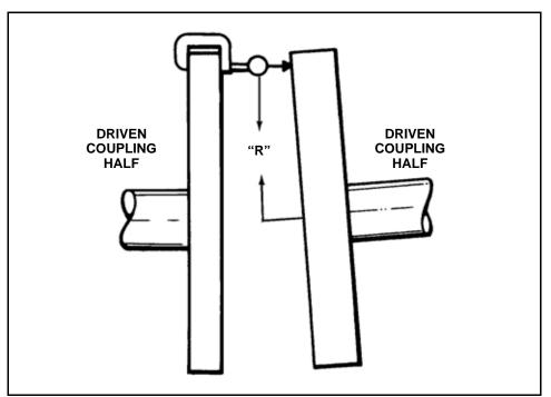
Figure 3-34 Measuring Angular Alignment
