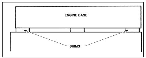
Figure 3-20 Level Engine Base With All Natural Sag Removed
