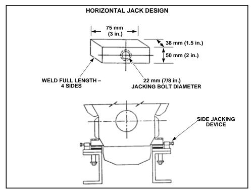
Figure 10-7 Jacking Devices
