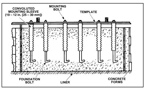
Figure 2-10 Mounting Sleeves Embedded in Concrete
