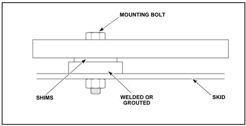
Figure 10-2 Shimming an Engine
