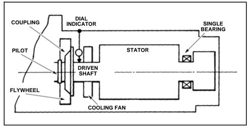
Figure 3-24 Single Bearing Generator
