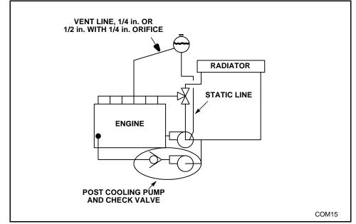
opening the thermostat. This allows warm bypass water to blend with the cooler return water which slowly cools the engine and closes the thermostat.
