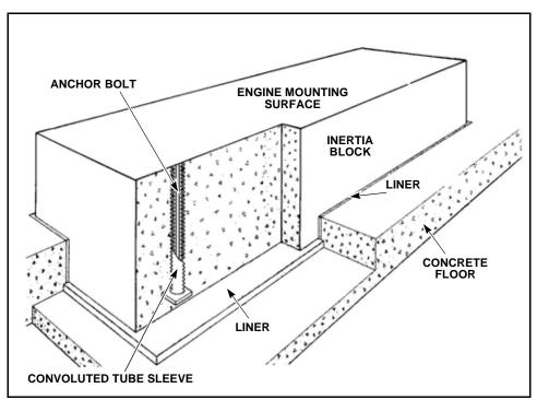
Figure 2-5 Cross Section of Concrete Inertia Block
