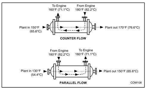
Figure 5-3 Counter and Parallel Flow Heat Exchanger
