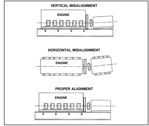
Figure 10-6 Angular Alignment
