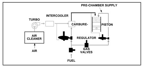
Figure 9-4 Pre-Chamber Lean Combustion Engine (Blow-Thru)
