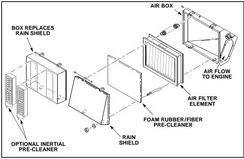
Figure 7-3 Typical Air Cleaner Components
