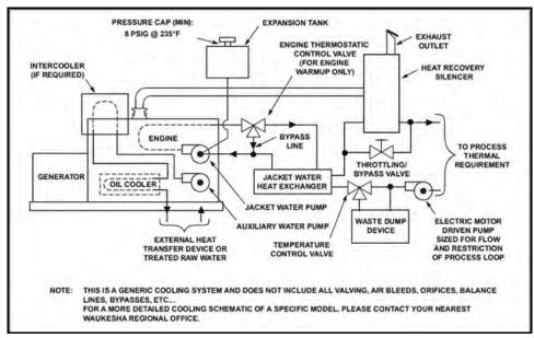
Figure 5-20 Isolated Circuit Heat Recovery System
