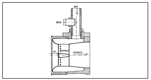
Figure 9-6 Venturi Type Carburetor
