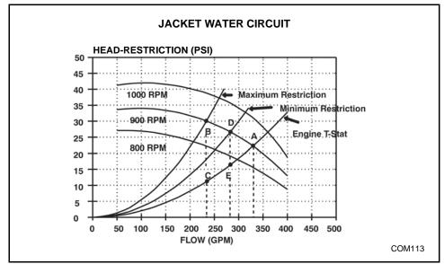
Figure 5-8 Water Pump Curve with Minimum Restriction
