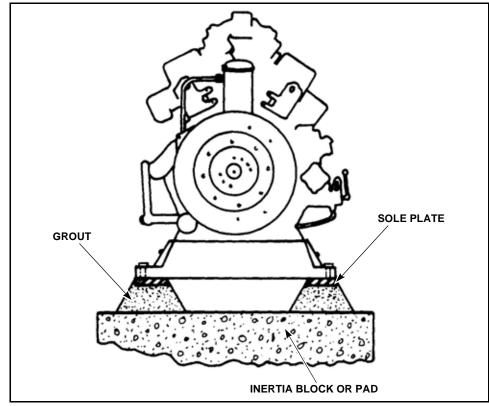
Figure 2-13 Rear View of Mounted Engine
