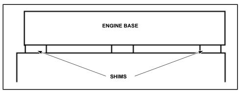
Figure 3-12 Level Engine Base with Natural Sag Removed
