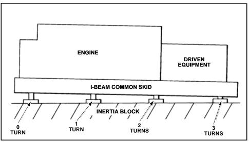
Figure 3-17 Leveling Spring Isolators
