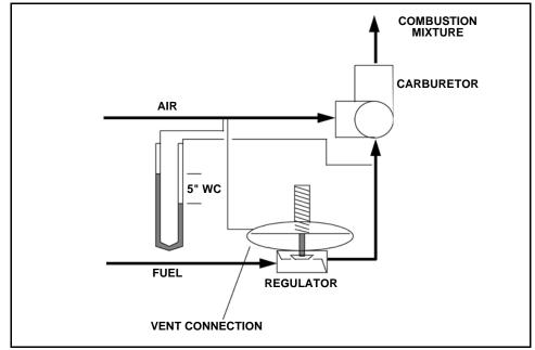
To account for these pressure variances, the regulator vent port is connected near the air inlet side of the carburetor.
