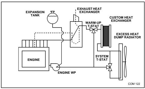
Figure 5-18 Single Pump Heat Recovery System (vent lines not pictured)
