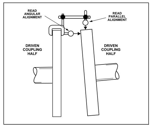
The amount of parallel misalignment is one-half the TIR (total indicator reading) for each direction.
