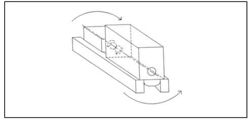
Figure 10-10 Torsional Rigidity in Skid
