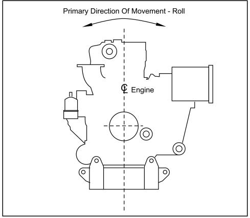
Figure 4-1 Primary Movement of an Engine
