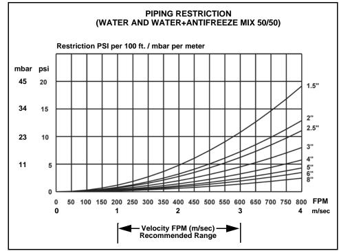
2. Determine pressure loss (P<sub>L</sub>) per 100 ft or meter of pipe for the velocity and pipe size from Figure 5-10.
