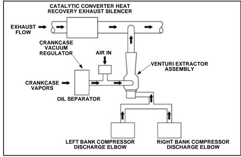
Figure 6-5 Ejector Type Systems (Optional)
