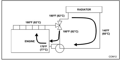
Figure 5-21 Thermostat Partially Open
