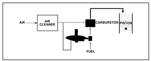
Figure 9-1 Naturally Aspirated Engine
