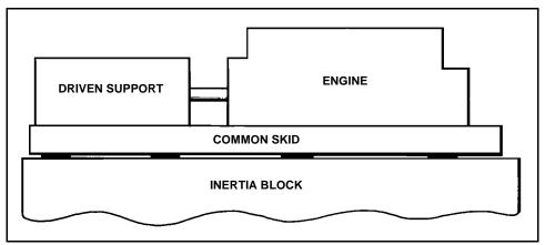
Figure 2-1 Engine and Driven Equipment on Common Skid
