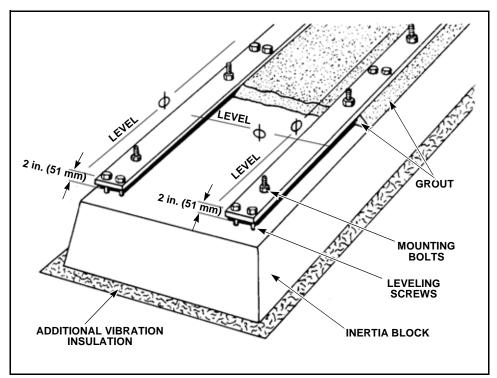
Figure 2-12 Grouting the Inertia Block
