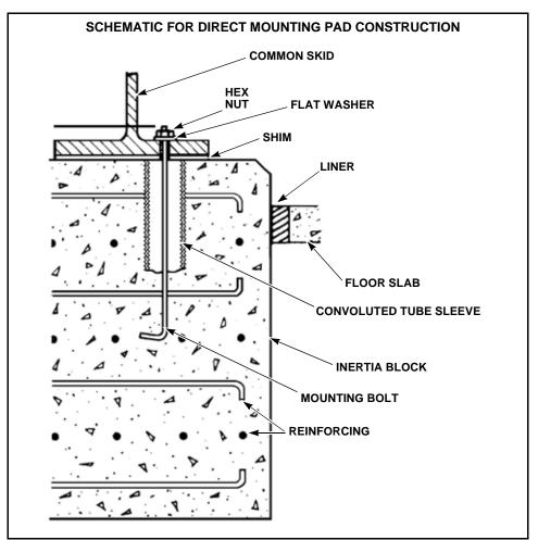
Figure 2-4 Common Skid Mounted Directly to Inertia Block or Pad
