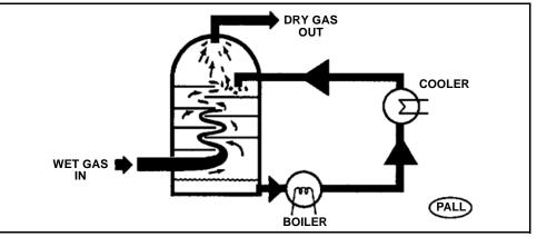
Absorption works well for water removal but is not suitable for removal of liquid hydrocarbons or compressor oil carryover.
