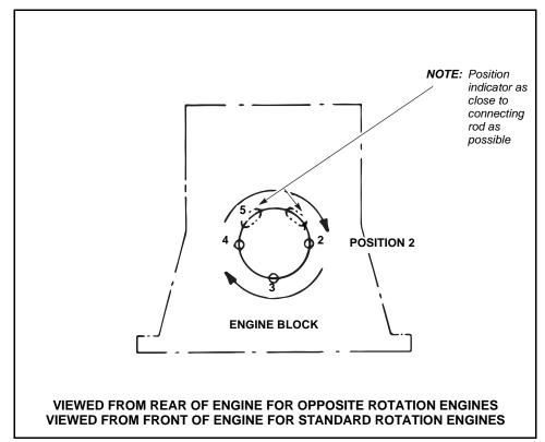
Figure 3-22 Location for Checking Crankshaft Deflection
