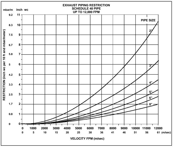
Figure 8-2 Restriction vs. Velocity for Pipe Diameter Up to 8 in.
