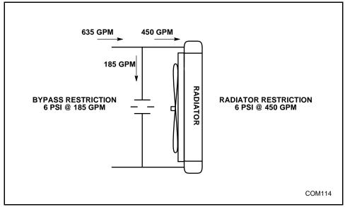
Figure 5-9 Cooling System with Bypass Pipe
