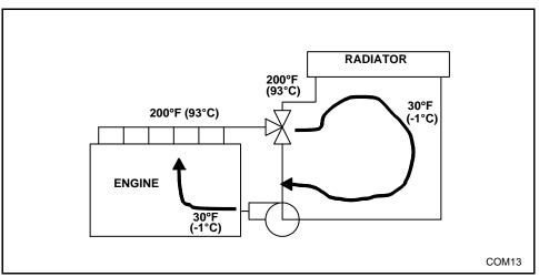
Figure 5-22 Thermostat Fully Open
