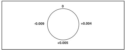
Figure 3-27 Total Indicator Reading (TIR)
