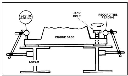
Figure 3-10 Record the Right Free Corner Indicator Reading
