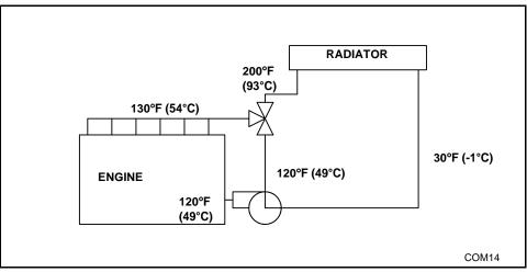
Figure 5-23 Thermostat Fully Closed
