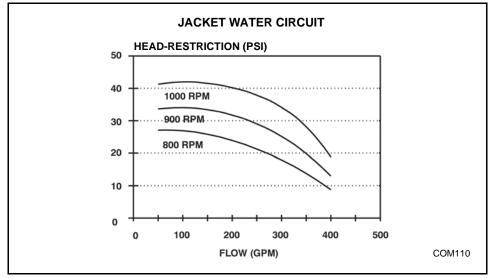
Figure 5-5 Water Pump Output
