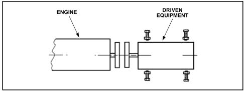
Figure 10-15 Correct Angular Alignment
