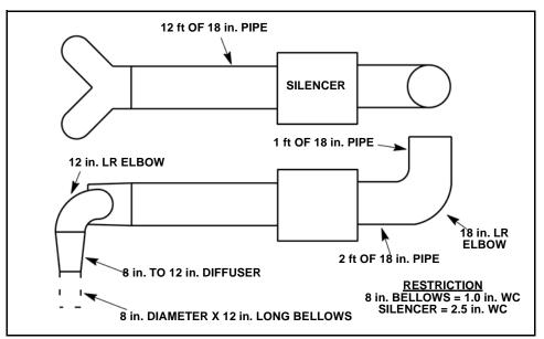
Figure 8-6 Schematic for Sample Problem
