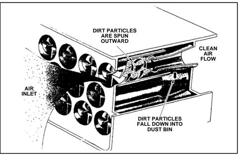
Figure 7-2 Inertial Type Precleaner
