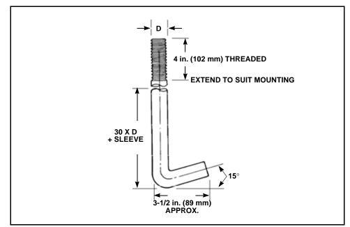
Figure 2-8 Mounting Bolt
