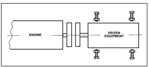
Figure 3-42 Correct Angular Alignment
