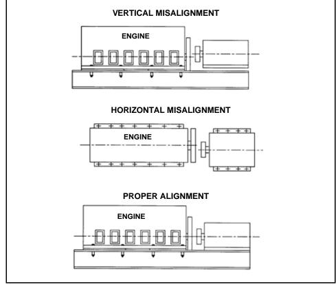
Figure 10-16 Parallel Alignment
