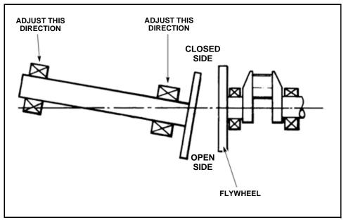
Figure 3-38 Make Adjustment to Close the Open Side of the Coupling
