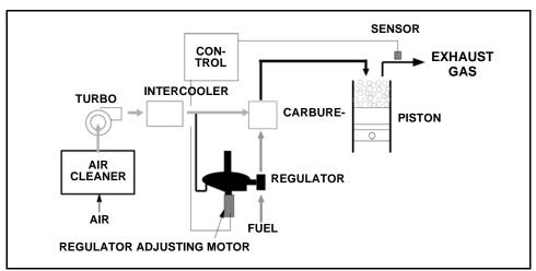
Figure 9-5 Electronic Air/Fuel Ratio Control
