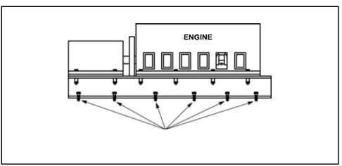
Figure 10-20 Adjust for Minimum Crankshaft Web Deflection per Section
