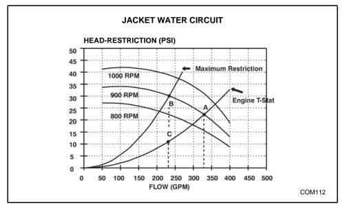
Figure 5-7 Water Pump Curve with Maximum Restriction
