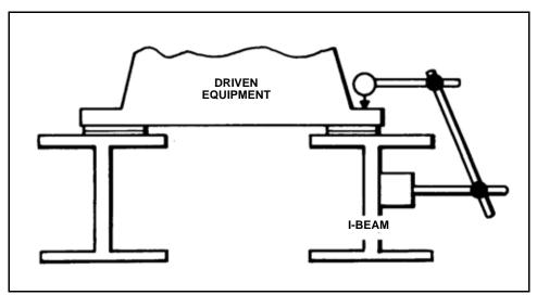
Figure 3-23 Driven Equipment Base Deflection
