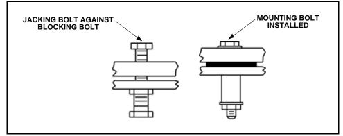
Figure 10-5 Jacking Using Mounting Bolt
