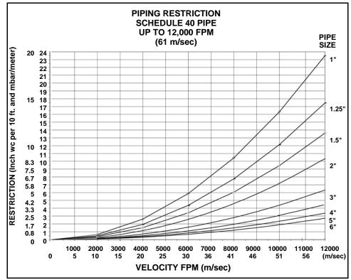
Figure 9-16 Restriction vs. Velocity for Pipe Diameters Up to 6 in
