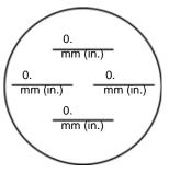
6. Check and adjust parallel alignment. Maximum TIR 0.127 mm (0.005 in.).
