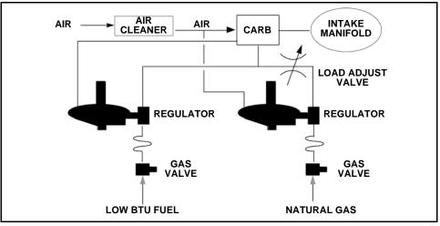
Figure 9-8 Single Carburetor
