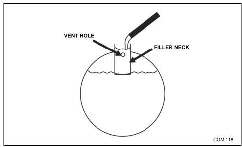
Figure 5-14 Vent Hole in Filler Neck
