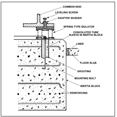
Figure 2-6 Schematic Spring Isolator Mounting Pad Construction
