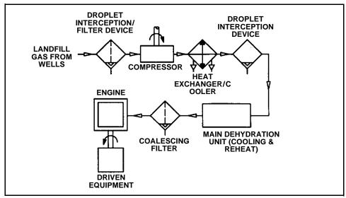
Figure 9-14 Typical Landfill Gas Fuel Treatment System
