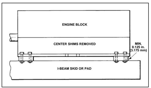
Figure 3-8 Corner Lift Method
