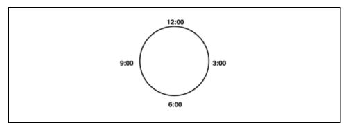
Figure 10-8 Dial Indicator Reading Positions When Measuring Angular Alignment
