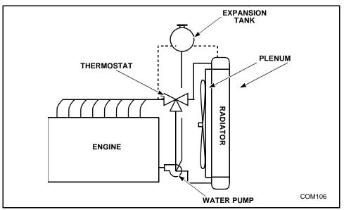
Radiators are typically used when an application has no use for the engine heat, so it is dumped to the ambient air.
