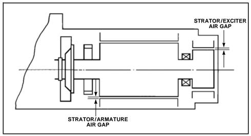
Figure 3-32 Single Bearing Generator
