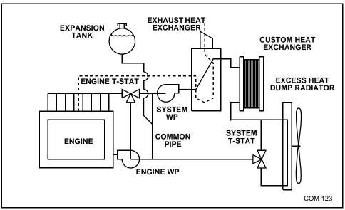
Figure 5-19 Two Pump Heat Recovery System (vent lines not pictured)
