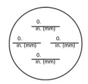
8. Check and adjust angular alignment. Maximum 0.005 in. (0.127 mm) TIR at flywheel bolt.
