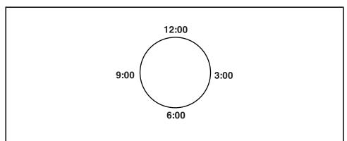
Figure 3-26 Dial Indicator Reading Positions When Measuring Angular Alignment
