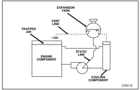
Figure 5-12 Schematic of Cooling Circuit
