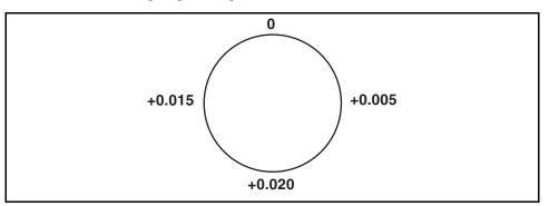
Figure 10-18 Total Indicator Reading (TIR)
