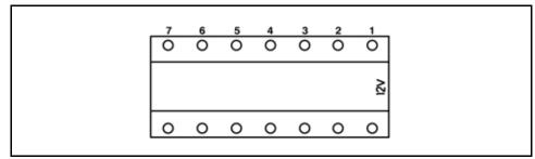
Figure 10-4 Bolt Locations for 12-Cylinder Model
