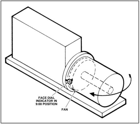
Figure 3-30 Dial Indicator Positioning
