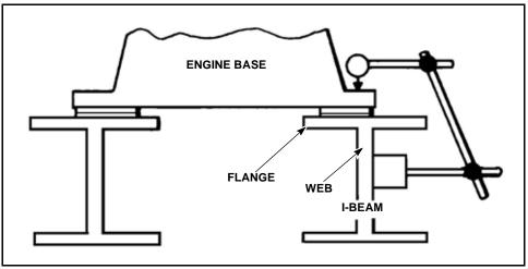
Figure 3-5 Correct Mounting
