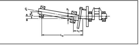
Figure 10-10 Multi-bearing Driven Equipment
