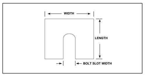
Figure 10-1 Shim Schematic
