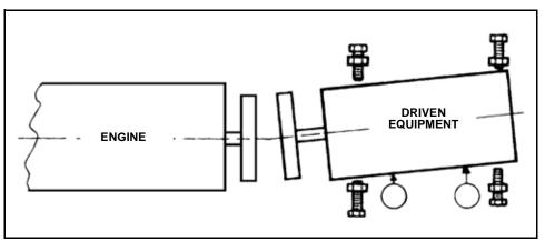
Figure 3-39 Indicator Positioning
