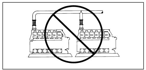
Figure 8-7 Common Exhaust System
