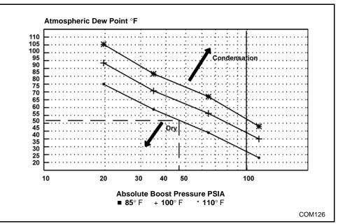
Figure 5-25 Boost Pressure vs. Dew Point to Determine Intake Manifold Condensation
