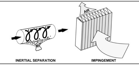
Figure 7-1 Air Filtration by Inertial Separation and Impingement
