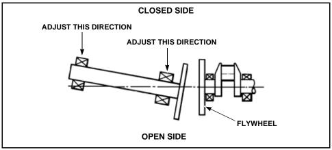
Figure 10-11 Adjusting Coupling
