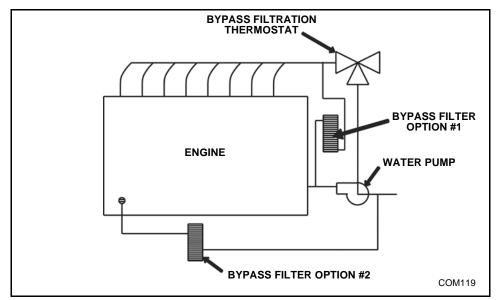
Figure 5-15 Schematic for Bypass Water Filtration Systems
