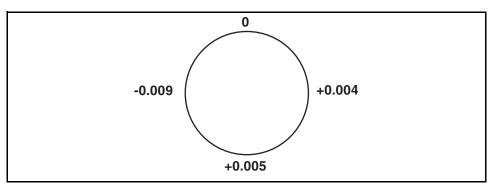
Figure 10-9 Total Indicator Reading (TIR)
