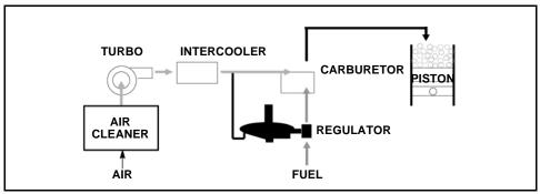
Figure 9-2 Turbocharged Engine
