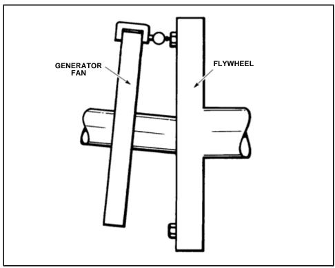
Figure 3-25 Angular Alignment-Single Bearing Generator
