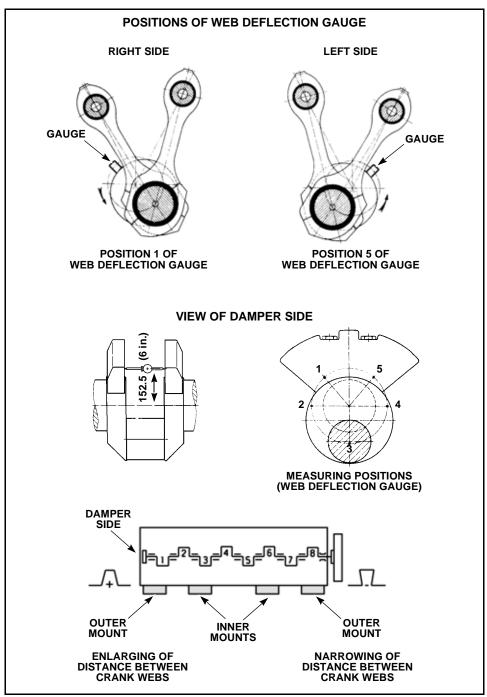
Figure 10-5 Checking the Crankshaft Deflection
