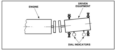
Figure 10-12 Adjusting for Angular Alignment
