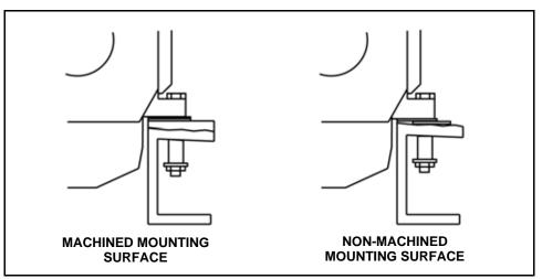
Figure 10-1 Machined Surface Mounting
