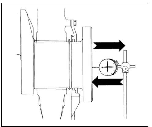
Figure 3-31 Checking Crankshaft Endplay
